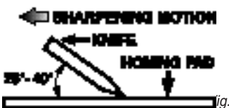
correct angle and motion Fishhook Sharpening Pad
