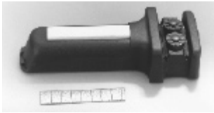
Fig. 3: Auxiliary honing pad (on handle) and coarse diamond pad Honing Pad
